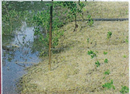
Figure 38. Nov 05. Rope 100mm above cleared topsoil stretched between stakes to measure the occurrence of erosion along foreshore of saltwater tidal creek (note black poly water pipe).
