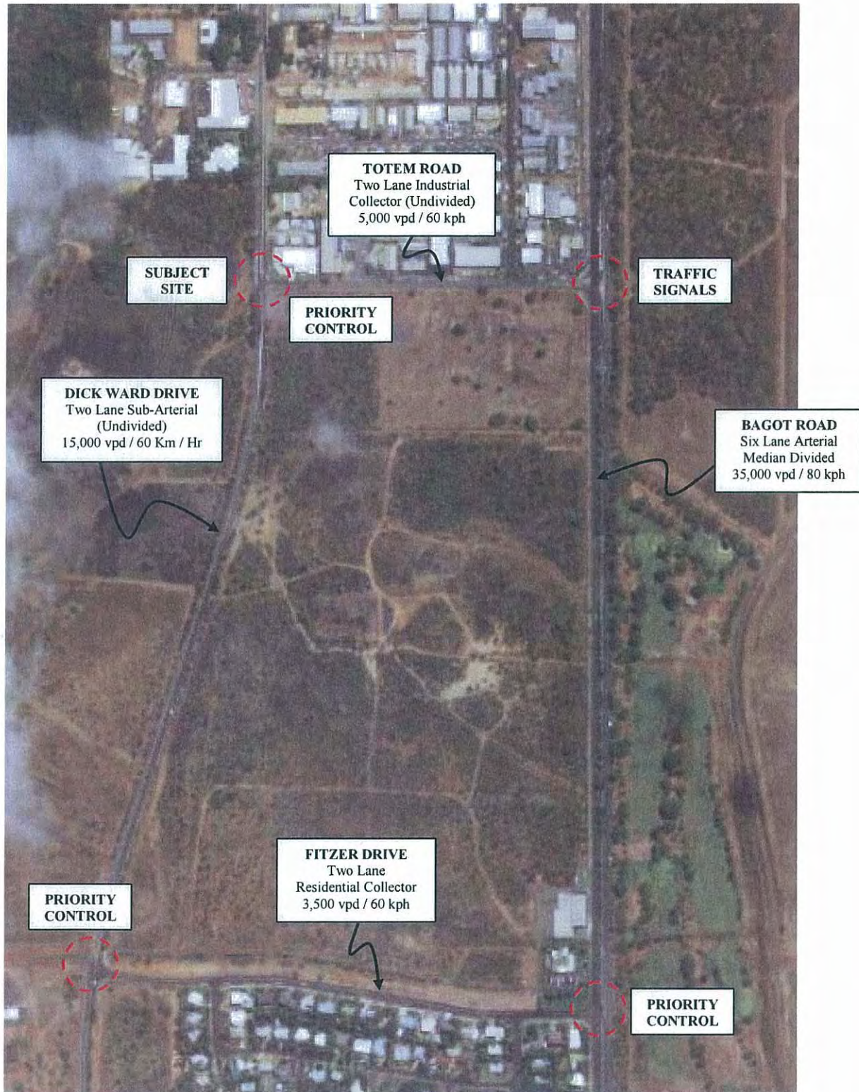
FIGURE 4.1 – ROAD NETWORK CHARACTERISTICS
